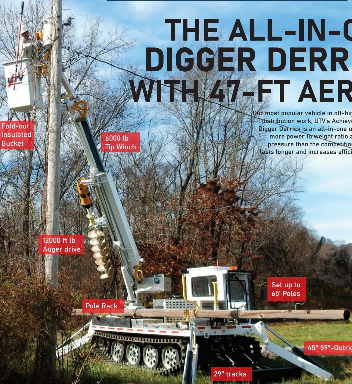
Our most popular vehicle in off-highway power line distribution work, UTV's Achiever RT-02 Tracked Digger Derrick is an all-in-one utility vehicle with more power to weight ratio and lower ground pressure than the competition. It goes further, lasts longer and increases efficiency and uptime.
